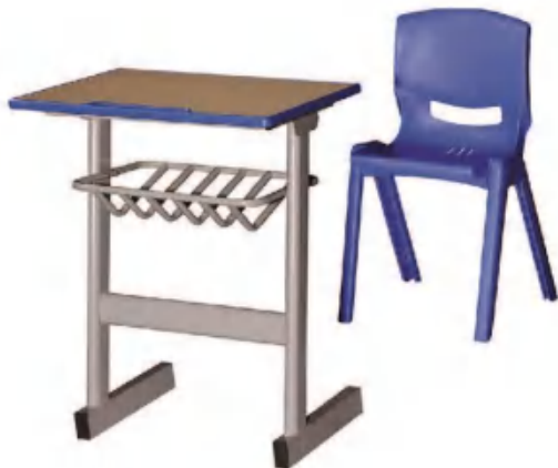
NJ-02702 单人课桌椅 Table size:600x400x750mm top:MDF 18mm frame:steel 1.2mm Chair seat:PP
